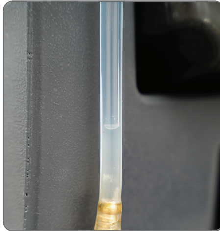
Clean water level indicator
