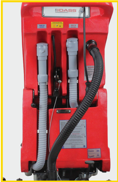
Water Drainage Hoses
