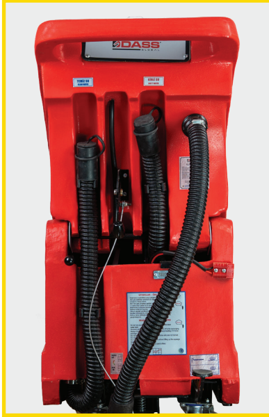
Water Drainage Hoses
