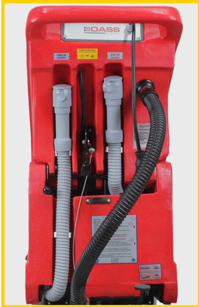
Water Drainage Hoses
