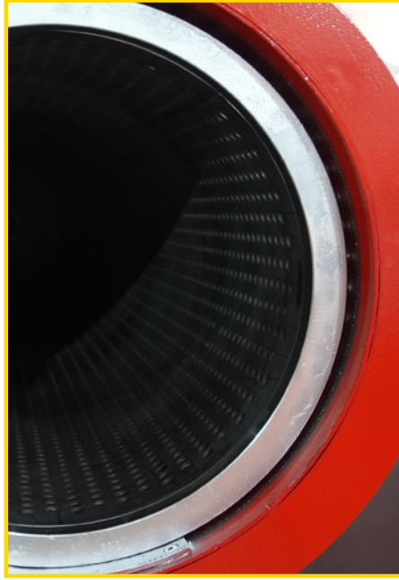
304 Quality Stainless Steel 3 mm Drum Thickness
